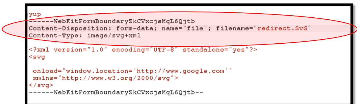
Figure 12 Change the Content-Type and Extension of the File
